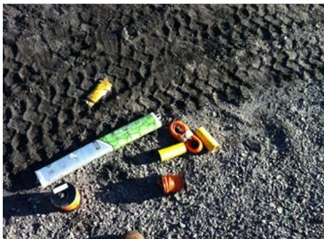
**Image 1. Crushed booster close to detonator and other accessories**
